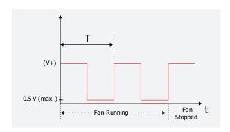
Open Collector Tachometer "FG" output voltage waveforms
