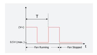
**Tacho Frequency** RPM=60/2T=30 f (f=frequency)
